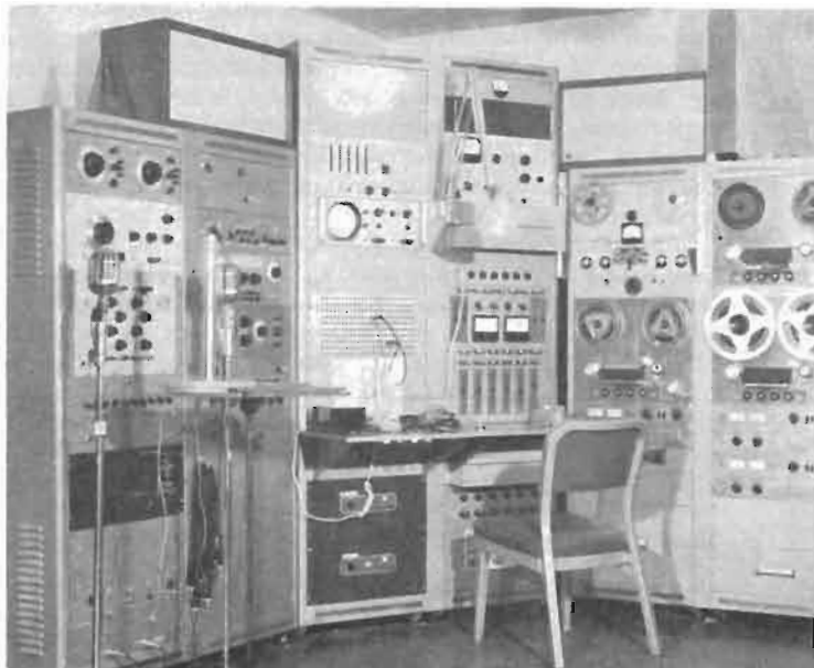
Fig. 2. University of Illinois Experimental Music Studio. Generating and processing equipment is on left, mixing and routing controls are in center, and the recorders are at the right.
