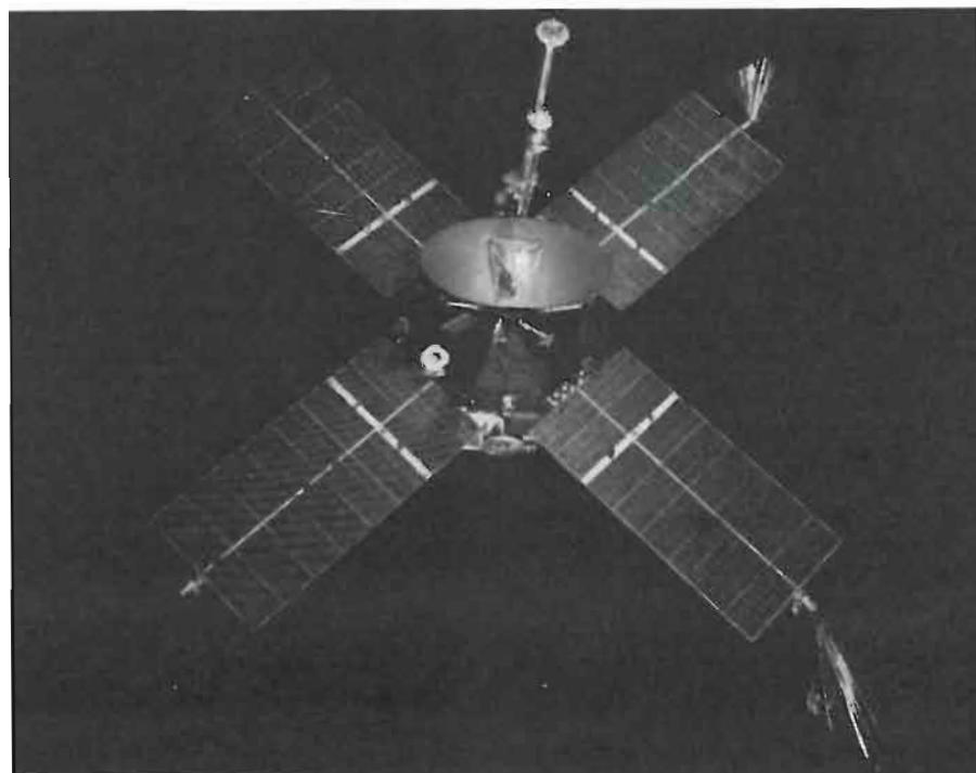
Satellites such as Mariner IV have a more complicated radar signature on account of the solar-cell paddles that are used.
