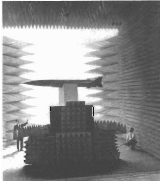
The target end of Bunker-Ramo Corp.'s microwave anechoic chamber. Foam plastic pyramids lining chamber absorb radiation.
